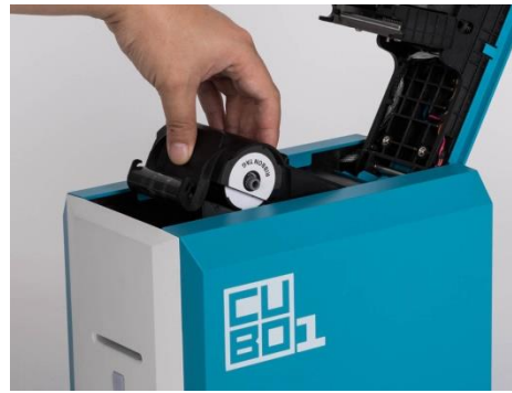
Figure 15 Installing the ribbon cartridge
